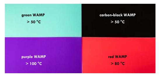
When the WAMP is heated up to the release temperature it expands to approx. 300  $\mu m$  thickness causing the release of the parts.
